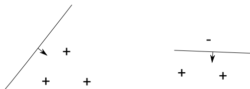
Figure 10.1.3: With three points, there are two types of configurations: collinear or noncollinear. Noncollinear configurations can be shattered.
