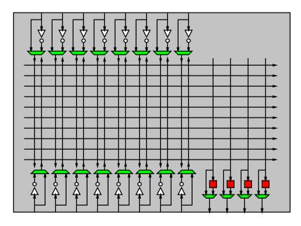
*N.B.* I think of the 8b-ALU logic block and PLA as being roughly the same size. The 4-LUT cascade logic block is about one-fourth the size of the PLA or 8b-ALU. This is the reason for the different distance metrics.
