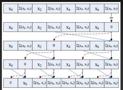
$$\begin{split} x[n-1] &= 0\\ \text{for } d &= \log_2(n) - 1 \text{ down to 0 do}\\ \text{for all } k &= 0 \text{ to } n-1 \text{ by } 2^d+1 \text{ in parallel do}\\ t &= x[k+2^d-1]\\ x[k+2^d-1] &= x[k+2^d]\\ x[k+2^d] &= t+x[k+2^d] \end{split}$$
